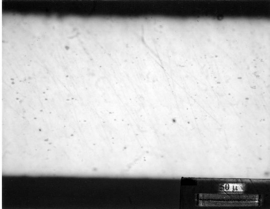
Figure 4: Microstructure of the edge of the copper tape taken from a new and unused cable. (Mag. 500X)
